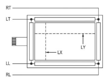
Loop Resistance X = short RT and RL, short LT and LL, measure the resistance between RT and LT Loop Resistance Y = short RT and LT, short RL and LL, measure the resistance between RT and RL
