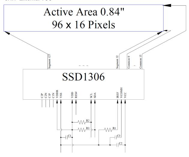
Pins connected to MCU interface: RES#, SCL and SDA
