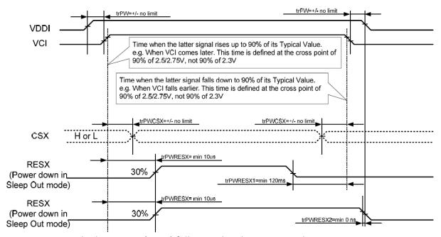
trPWRESX1 is applied to RESET (RESX) falling in the Sleep Out Mode trPWRESX2 is applied to RESET (RESX) falling in the Sleep In Mode
