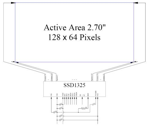
MCU Interface Selection: BS1 and BS2 Pins connected to MCU interface: D7~D0, E/RD#, R/W#, D/C#, RES# and CS#.
