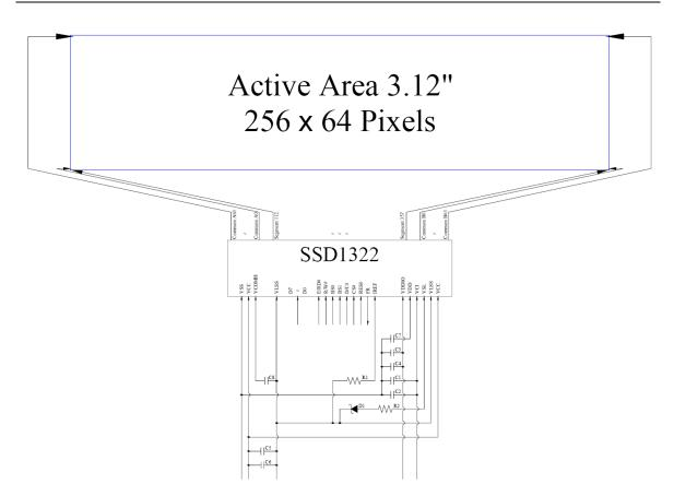
MCU Interface Selection: BS0 and BS1 Pins connected to MCU interface: D7~D0, E/RD#, R/W#, D/C#, CS#, and RES#
