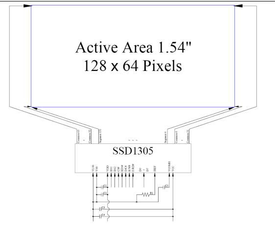
MCU Interface Selection: BS1 and BS2 Pins connected to MCU interface: D7~D0, E/RD#, R/W#, D/C#, RES# and CS#.
