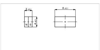
Magnet for direct application onto customer's shaft (see user manual).
