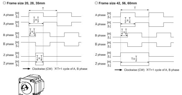
%It is recommended to use Line driver output (corresponding to 26C32) at RECEIVER end of encoder output and terminating resisters (100-150Ω) in parallel at both ends of each phase (A, A, B, B, Z, Z, corresponding to 26C31).
