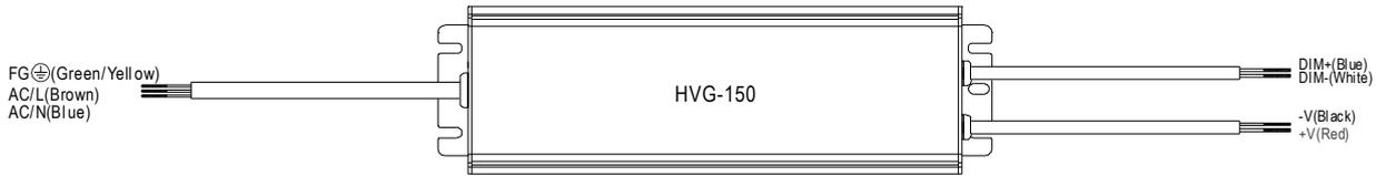
※ Built-in 3 in 1 dimming function, IP67 rated. Output constant current level can be adjusted through output cable by connecting a resistance or 0 ~ 10V dc or 10V PWM signal between DIM+ and DIM-.
