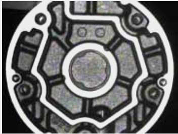
Surface reflectivity difference between the machined aluminum and cast aluminum (direct vs. scattered light)
