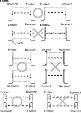
• Baffle should be installed between 2 sets.
