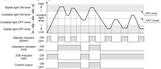
XThe waveforms of operation indicator, job indicator, and control output are the state of operation for Light ON, but in case of Dark ON, it is opposite operation against Light ON mode.
