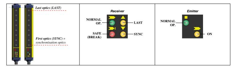
Signals are clearly identified through symbols allowing immediate reading, independent of bars directions. A short description of the signalling LEDs is necessary to avoid misunderstandings.
