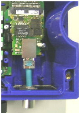
Figure 5 – Ethernet/IP Module – Modbus TCP Module IP65 Mounting
