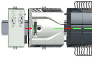
**6.** ➤ Rebind your modules by moving the CPU along with the extension module on the mounting rail.
