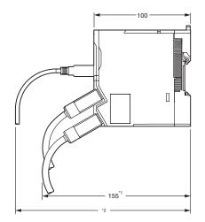
Note: 1. This is the dimension from the back of the unit to the communication cables: - 155 mm: When an XS6G-T421-1 connector is used.
