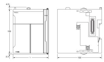
Note: 1. This dimension depends on the selected power supply unit: - 51 mm: NX-PD7001 - 80 mm: NX-PA9001
