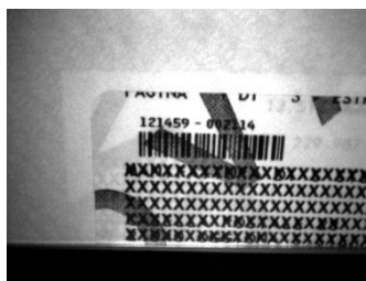
Figure 16 - Overprinted Barcode Readable by Matrix 300™ also Through the Envelope Window Film
