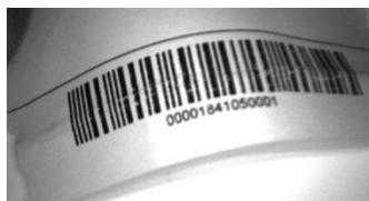
Figure 17 - Barcode Printed on Curved Surface Readable by Matrix 300™ in spite of Image Optical Distortion
