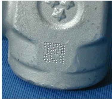
Figure 18 - Dot Matrix Code Directly Marked on Metal Surface by Using Dot Peening Technology
