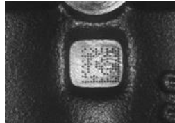
Dot Peening On Scratched Surface
