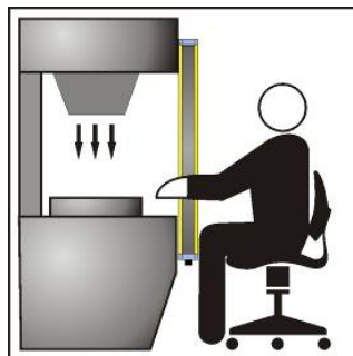
Fig. 8 Safety light curtain positioning
