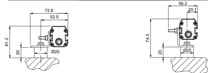
Standard bracket + antivibration support (ST-K 4/6 AV)
