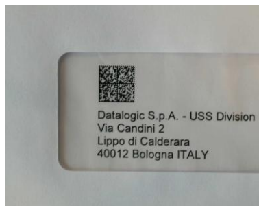
Figure 16 - Address Coded in Data Matrix Symbology for Automated Mail Processing
