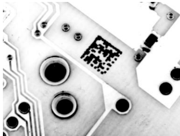
Figure 24 - Data Matrix Code Directly Marked on PCB Surface by Using Laser Etching Technology
