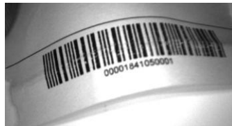
Figure 19 - Barcode Printed on Curved Surface Readable by Matrix 210™ in spite of Image Optical Distortion
