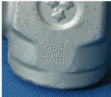
Figure 20 - Dot Matrix Code Directly Marked on Metal Surface by Using Dot Peening Technology
