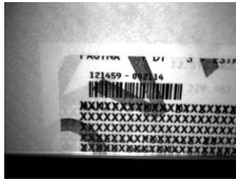
Figure 18 - Overprinted Barcode Readable by Matrix 210™ also Through the Envelope Window Film
