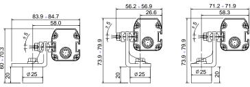
Plastic fixing bracket + Orientable support + Antivibration support
