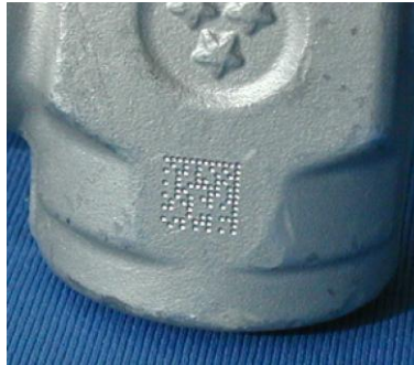
Figure 26 - Dot Matrix Code Directly Marked on Metal Surface by Using Dot Peening Technology
