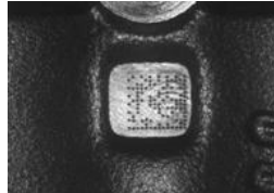
Dot Peening On Scratched Surface
