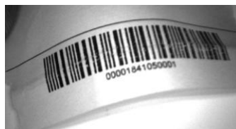
Figure 25 - Barcode Printed on Curved Surface Readable by Matrix 410™ in spite of Image Optical Distortion
