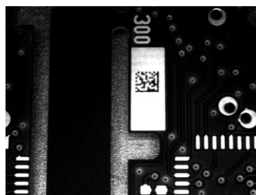
Figure 29 - Dot Matrix Code Directly Marked on PCB Copper Pad by Using Ink-Jet Technology
