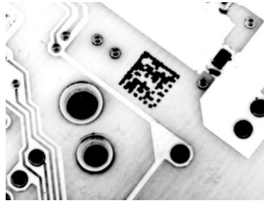
Figure 30 - Data Matrix Code Directly Marked on PCB Surface by Using Laser Etching Technology
