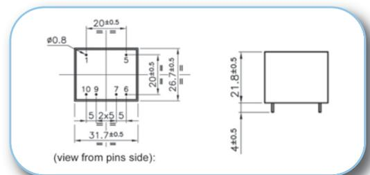
**DIMENSIONS and PINOUT**
