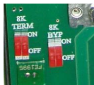
Figure 22 - PWO DIP Switch Settings
