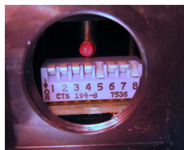
Standard encoder dip-switch setting "Encoder Step" = 252 (mm/100)
