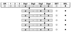
At each pressure of the SEL pushbutton, the different delay levels in ms are visualised in a cyclical manner at the output deactivation and moreover, the relative delay value will be stored. When the "d-00" message is visualised the operating mode will be "run", and "rund" in all other cases.
