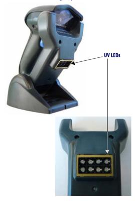
The Counterfeit Detector is based on UV fluorescent emission. Real banknotes under ultraviolet rays usually absorb the UV light and will show special marks made with fluorescent inks. However, most counterfeit banknotes only reflect the UV lights, without showing fluorescent marks.
