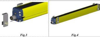
Insert the transparent plate and slide it along the binary under the fixing brackets. Once positioned correctly, tighten the screws with the N° 8 key, pressing the fixing bracket on the plate, until all the fixing brackets are blocked safely.
