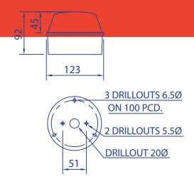
Compact xenon strobe visual warning device featuring ABS base and polycarbonate dome lens. Bases available in White (standard) or Black whilst lenses are available in Red, Amber, Green, Blue or Clear.
