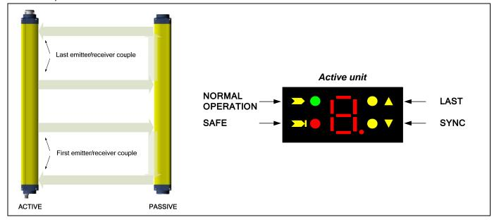
Signals are clearly identified through symbols allowing immediate reading, independent of bars directions. A short description of the signalling LEDs is necessary to avoid misunderstandings. Two yellow LEDs (▲ LAST, ▼ SYNC) on SG-BODY Reflector active unit, facilitate the alignment procedure.
