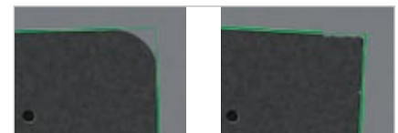
Edge and corner breakage inspection
