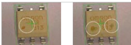
Inspection of scratches and defects
