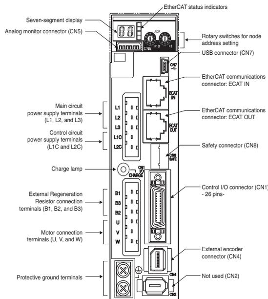
**Note:** The above picture shows 230 V servo drives models only. The 400 V servo drives have 24 VDC power input terminals for control circuit instead of L1C and L2C terminals.
