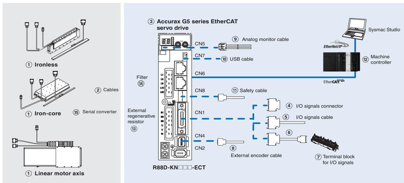
Note: The symbols ①②③④⑤... show the recommended sequence to select the components in Accurax G5 servo system
