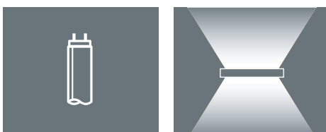
TYCOON fluorescent: Optimum quantity of direct light downwards and indirect light upwards.
