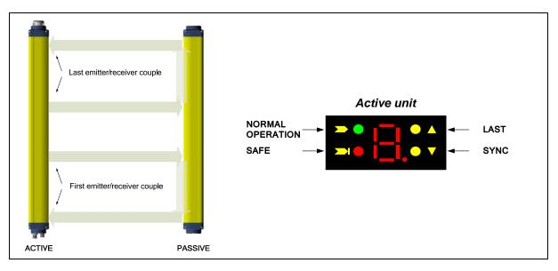
Signals are clearly identified through symbols allowing immediate reading, independent of bars directions. A short description of the signalling LEDs is necessary to avoid misunderstandings. Two yellow LEDs (▲ LAST, ▼ SYNC) on SG-BODY Reflector active unit, facilitate the alignment procedure.
