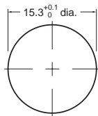
Panel Cutout Dimension Panel thickness = 1 to 4 mm
