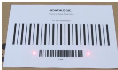
Figure 7 –Aligning the Focusing and PPI Setup Chart Using Laser Pointers as Reference
