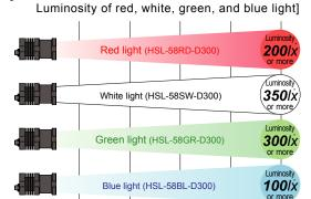
Maximum light intensity within the Ø300-mm diameter spot when it is illuminated with a 2,000 mm working distance from the front of the light. (The light intensity may vary with ambient temperatures.)
