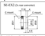
\*Insert between the lens and the camera mount to double the magnification. Note that nosity and resolution are reduced.
