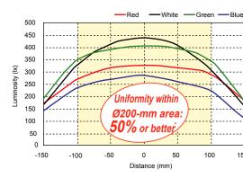
\* Light intensity value across the Ø300-mm spot diameter when it is illuminated with a 2,000 mm working distance from the front of the light.
