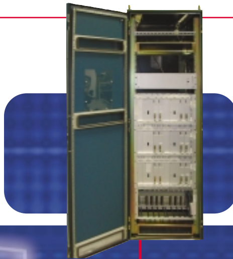
Computer based railway control centre (Photo: CSEE Transport)
