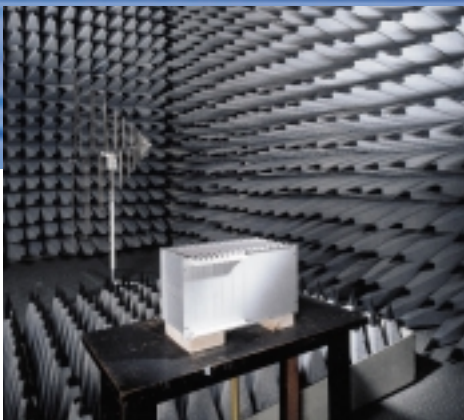
Gasketing concepts are tested in the laboratory at Karlsruhe University for EMC suitability
