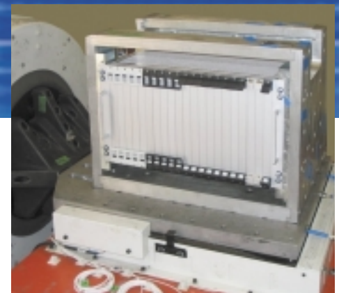
Subracks europacPRO during a shock and vibration test
